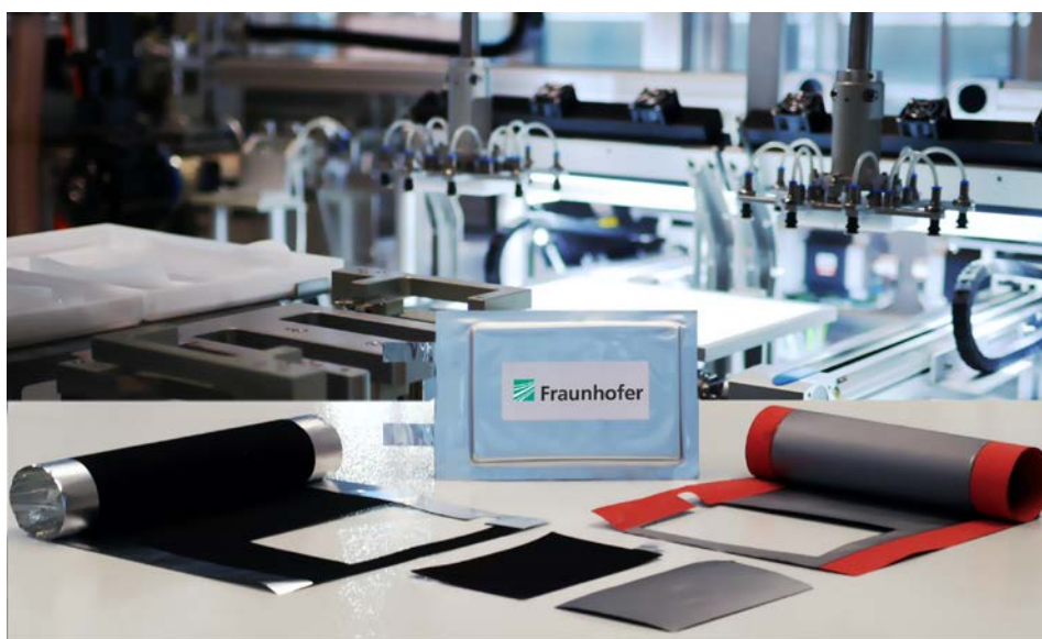
Lithium sulfur batteries: electrodes and prototype cells © Fraunhofer IWS Dresden
