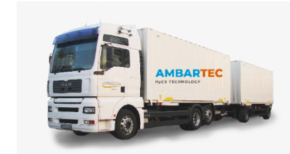
H 2 -Transport with AMBARtec 1 bar/1.200 kg H 2 /truck
